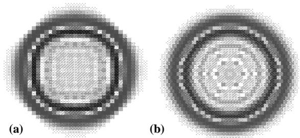
Figure 4. Wavefronts on, (a) rectilinear mesh, and (b) triangular mesh, 14 time steps after an applied Gaussian impulse.
