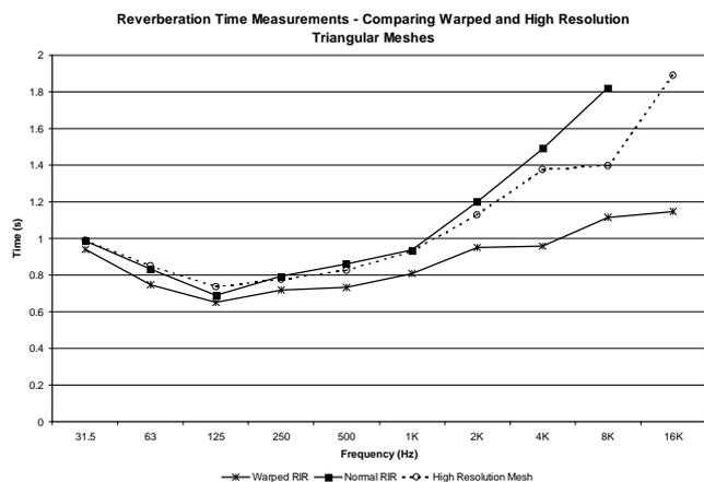
Figure 8. Reverberation Time measurements for the triangular, high-resolution triangular, and warped triangular mesh structures.
